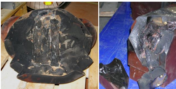
Figure 4. Examples of destruction of VIT with epoxy insulation
