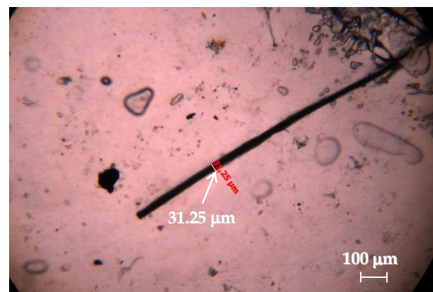
Figure 8. Result of measuring the diameter of the fuse-element of the SIBA fuse using an optical microscope
