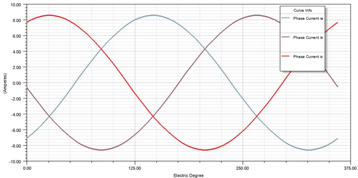
Figure 26. Winding Currents under Load
