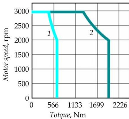
Figure 4. Load characteristics of EMG-10APA22: 1 - continuous working area; 2 - repeatedly working area
