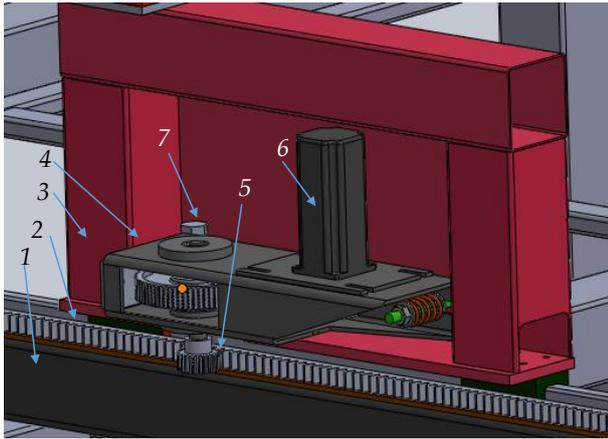
**Figure 1.** The main elements of the longitudinal drive to move the axis of the portal-type machine
