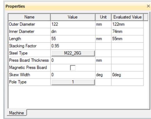
Figure 9. ANSYS RMxprt: stator core parameters
