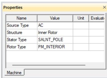
Figure 7. ANSYS RMxprt: global machine properties
