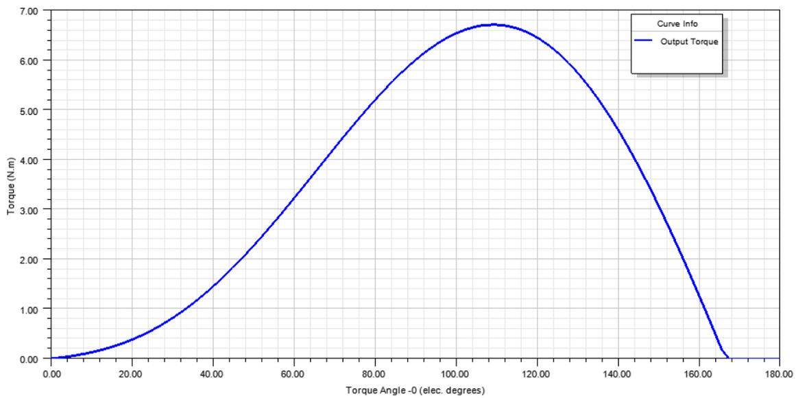
Figure 25. Output Torque vs Torque Angle
