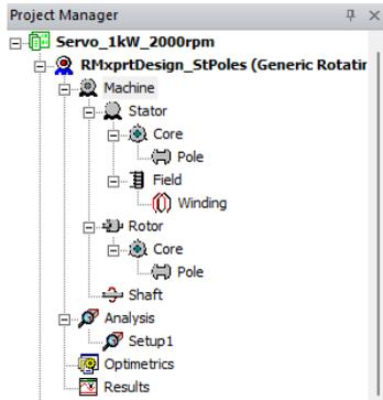
Figure 6. ANSYS RMxprt: machine characteristics tree
