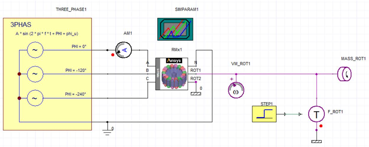
Figure 27. ANSYS Simplorer: simulated servomotor with a stable power supply
