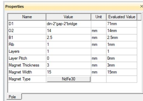
Figure 18. ANSYS RMxprt: permanent magnets dimensions
