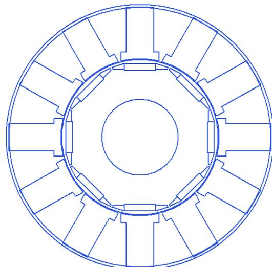
Figure 19. ANSYS RMxprt: servo motor sketch
