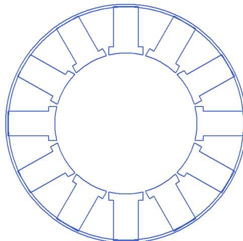
Figure 12. ANSYS RMxprt: sketch of a stator with poles
