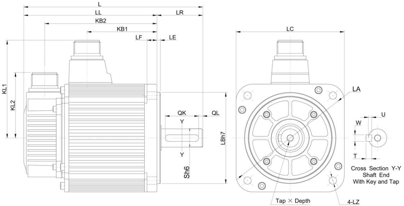
Figure 3. Servomotor EMG-10APA22 outline drawings
