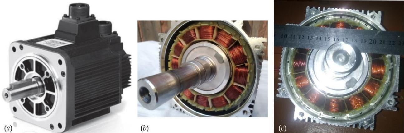
**Figure 2.** Views of the investigated servomotor: (a) – appearance of the EMG-10APA22 servomotor; (b) – servomotor with the endshield removed (experimental photo); (c) – view of the servomotor coils (photo of the experimental sample)
