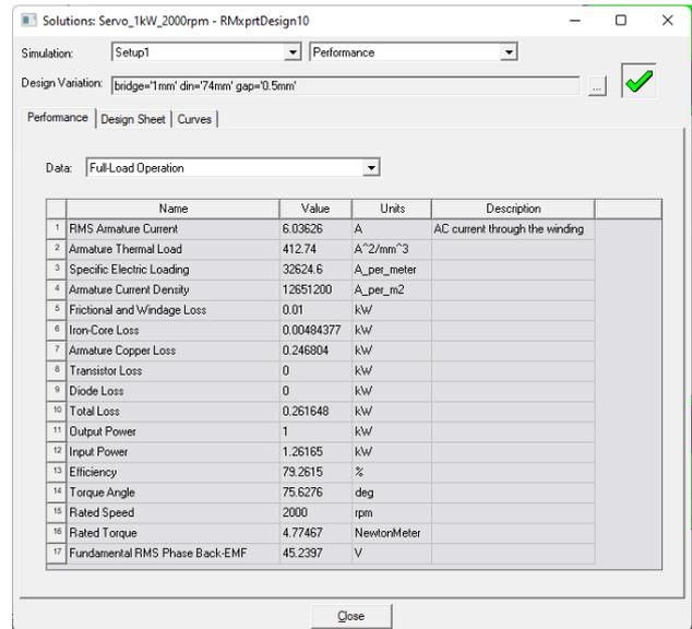
Figure 22. ANSYS RMxprt: Servomotor calculation report (data under load)
