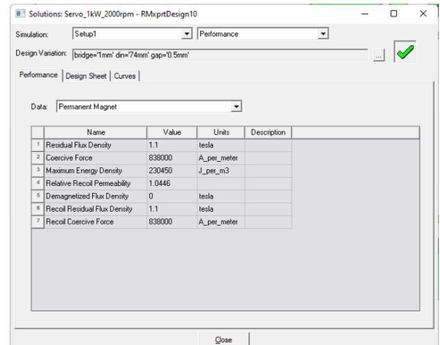
Figure 23. ANSYS RMxprt: permanent magnet solver report
