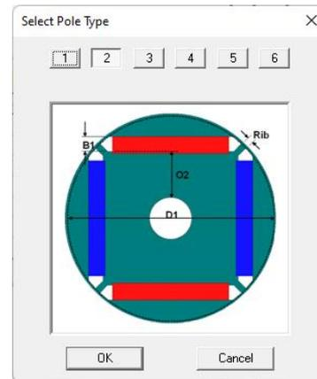
Figure 17. ANSYS RMxprt: selection of the permanent magnets type
