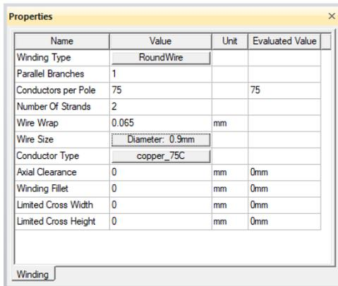
Figure 14. ANSYS RMxprt: winding parameters of inductors
