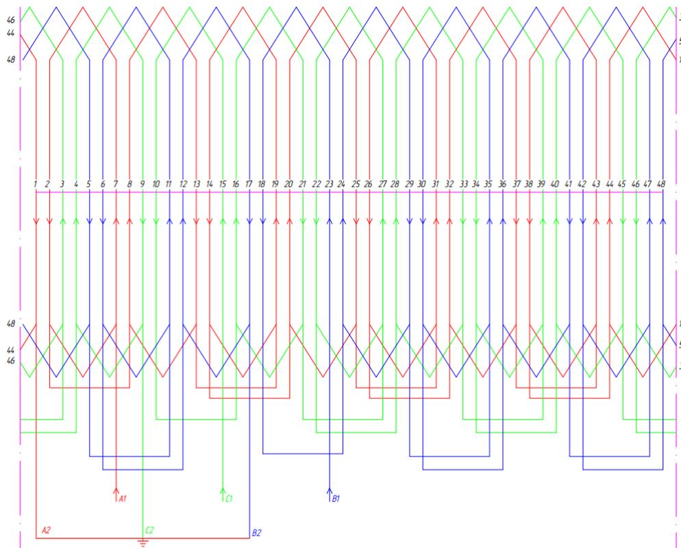
Figure 4. Scheme of the whole-coiled winding of the MFEC
