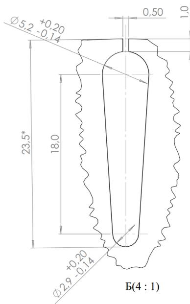
**Figure 6.** Sketch of the stator slot of the MFEC
