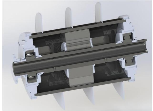
**Figure 2.** Longitudinal section of a screw-type multifunctional converter
