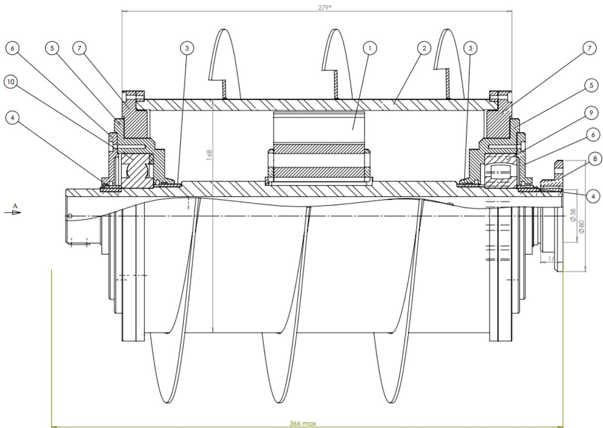
**Figure 3.** Assembly drawing of a screw-type multifunctional converter (view 1): 1 – stator; 2 – rotor; 3 – sleeve for the capsule; 4 – sleeve under the cover; 5 – capsule; 6 – cover; 7 – shield; 8 – flange; 9 – roller bearing; 10 – ball bearing
