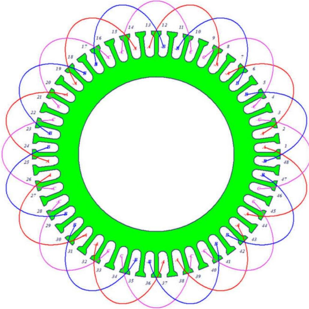
**Figure 5.** Sketch of the cross-section of the MFEC with winding in ANSYS RMxprt
