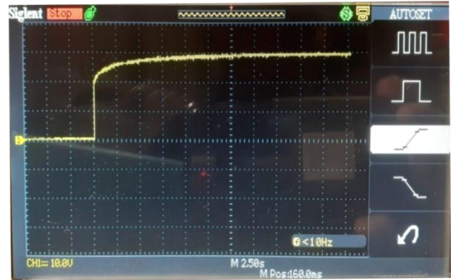
Figure 7. DC-DC converter output voltage change at load *20 kOhm (Input voltage 10 V, d = 50\% )
