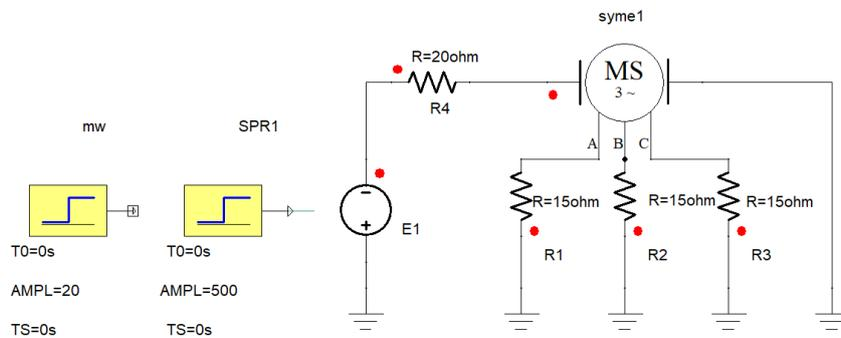
Figure 12. Simulation model of synchronous motor in ANSYS Twin Builder
