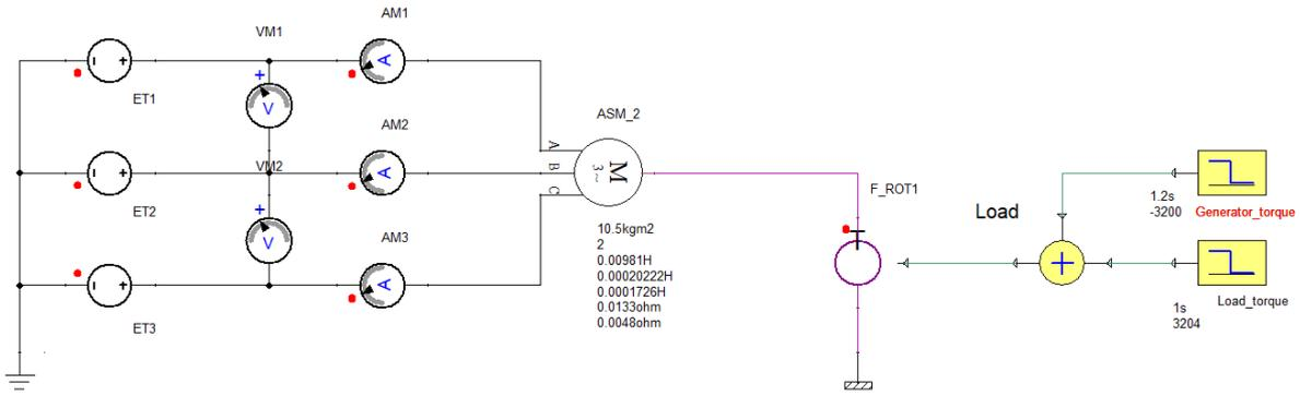
Figure 1. Simulation model of induction motor in ANSYS Twin Builder
