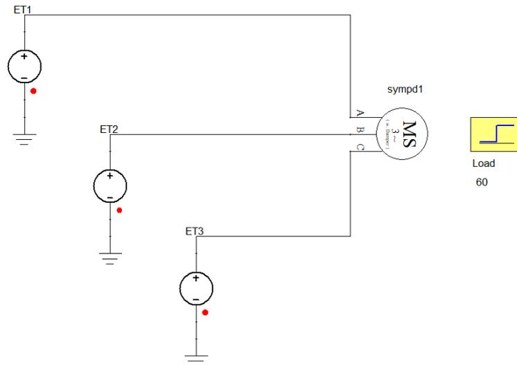
Figure 17. Simulation model of synchronous permanent magnet motor in ANSYS Twin Builder
