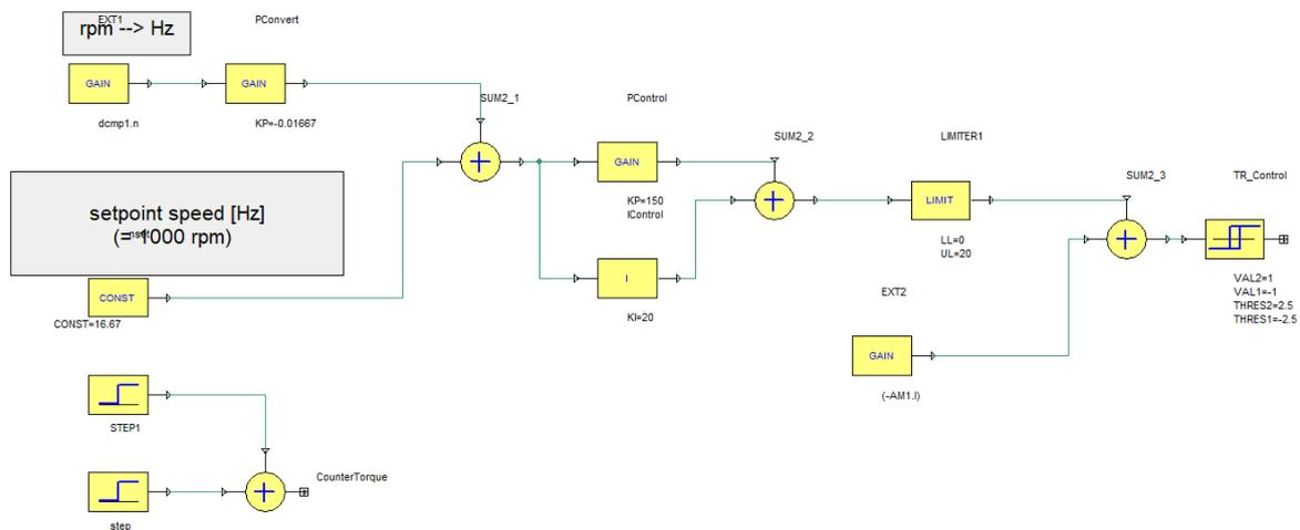
Figure 9. Simulation model of DC motor with permanent magnets in ANSYS Twin Builder: control part
