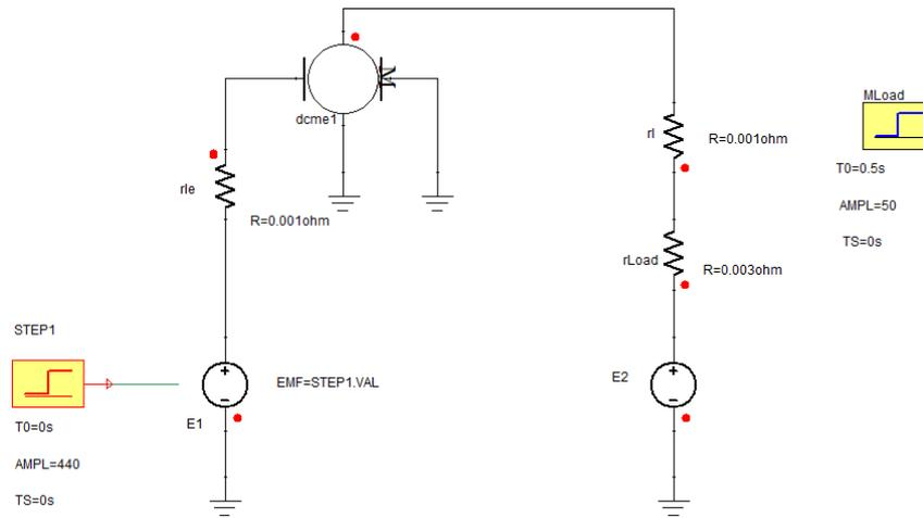
Figure 5. Simulation model of DC motor in ANSYS Twin Builder
