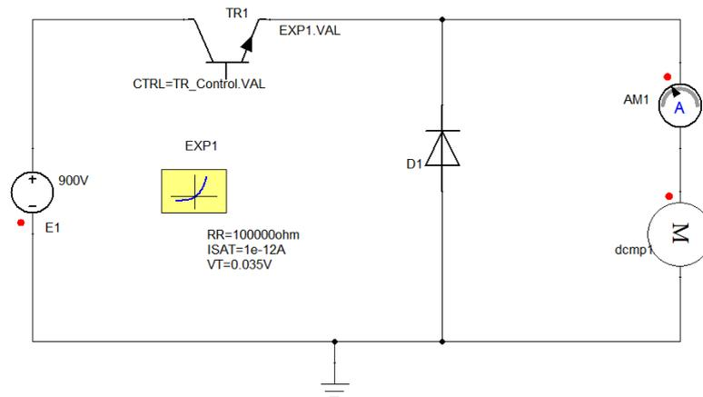
Figure 8. Simulation model of DC motor with permanent magnets in ANSYS Twin Builder: power part
